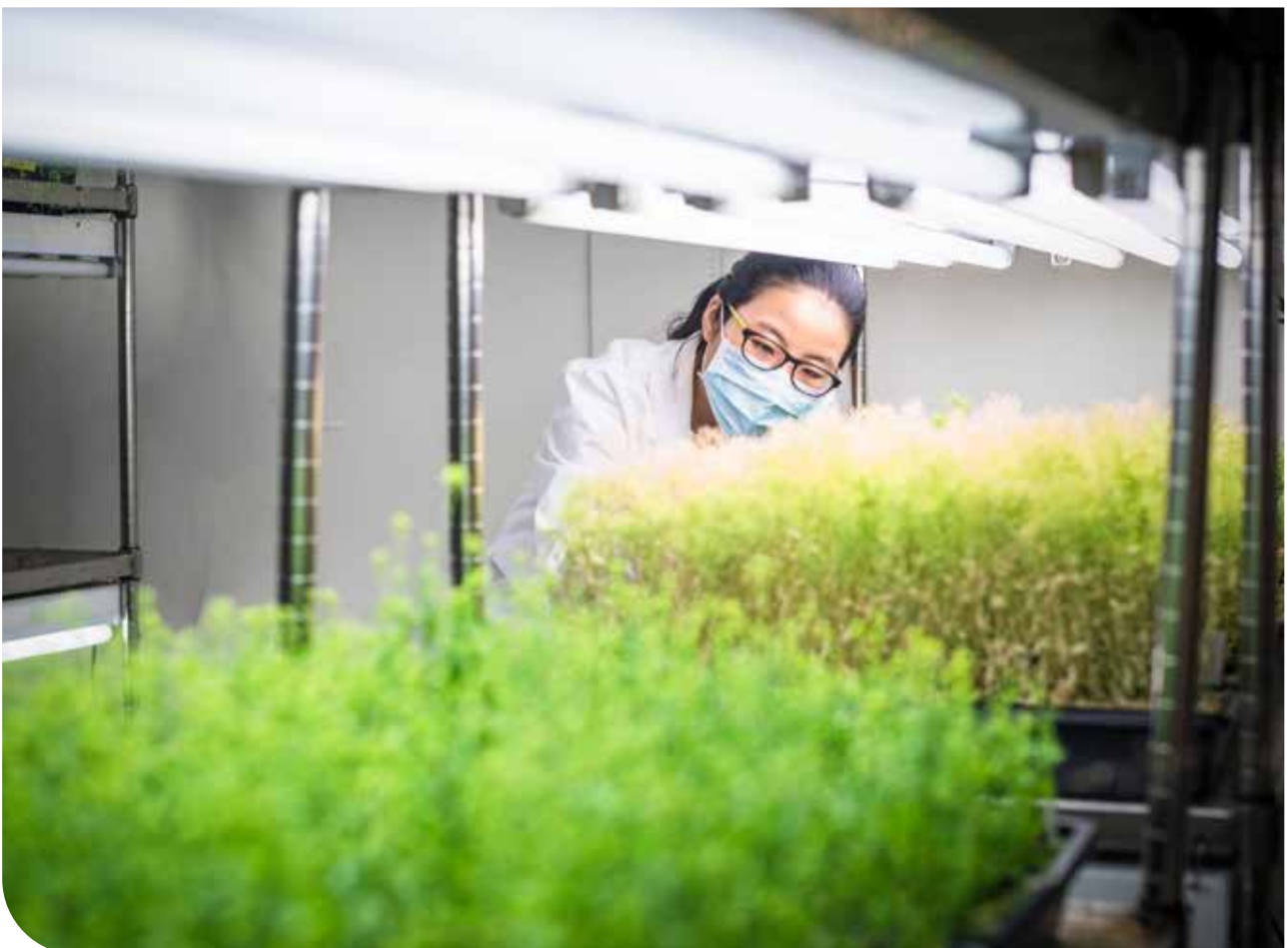
Fitotrone: controlled environment room, temperature and relative humidity adjustment, and photoperiod for quick agronomic screening
