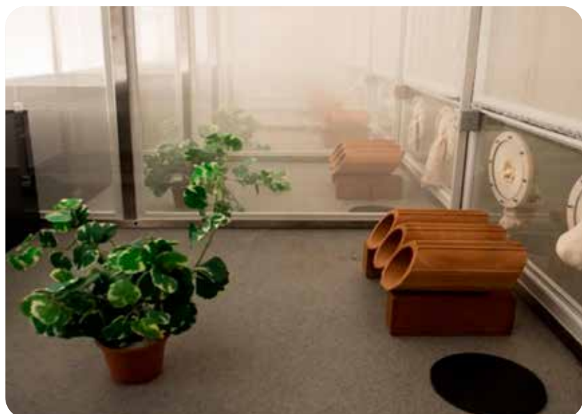
Temperature, humidity and photoperiod climatic room for the growth of entomological strains.
