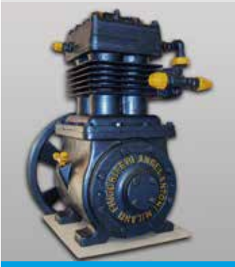
Double stage refrigeration compressor patented in 1949
